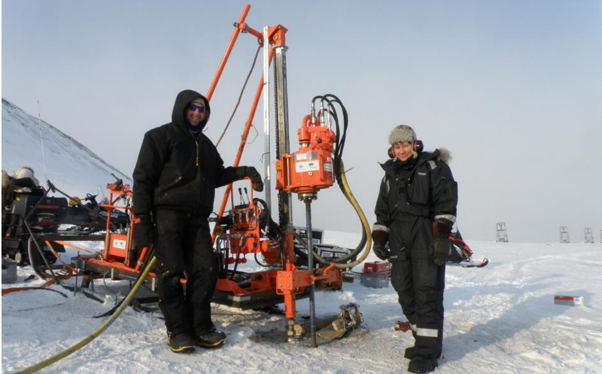
Betty drill rig collecting permafrost cores in Endalen outside Longyearbyen, being operated by Ulrich Neumann and with Hanne Christiansen. April 2012. (Photo: Ole Humlum/UNIS).
